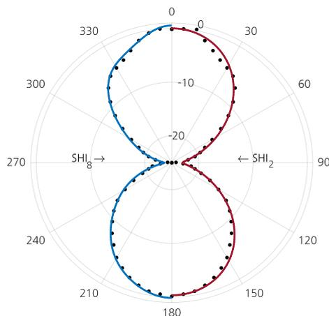
**Fig. 2:** Comparison of spherical harmonic interpolation computed with order limits of 2 and 8. While  $n \leq 2$  provides a smoother angular response,  $n \leq 8$  retains a higher level of detail. Measurement data: Schoeps MK8 at 10 kHz
