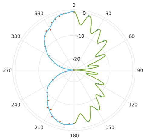
**Fig. 6:** Aliasing effects due to interpolation above the sampling limit. *Left:* Dataset with 72 measurement points in  $360^\circ$ , interpolated with  $n \leq 23$ . *Right:* Dataset with 24 measurement points in  $360^\circ$ , interpolated with  $n \leq 23$ . Choosing interpolation orders above the sampling limit introduces unwanted oscillations in the interpolated data. The higher the order, the more drastic the oscillations.
