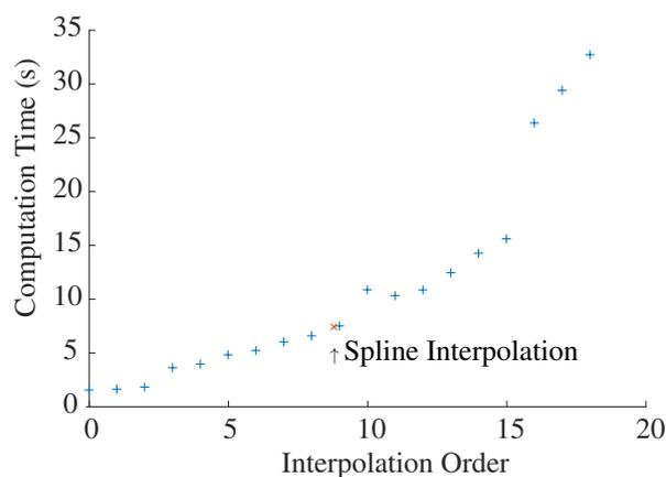
**Fig. 4:** Computational cost of interpolation algorithms. 24 Measurement points with 20000 frequency bins each were processed. Up to  $n = 8$ , spherical harmonic interpolation is faster than spline interpolation.
