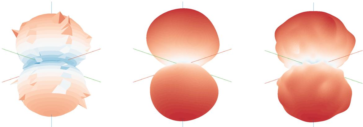
**Fig. 8:** Three-dimensional SHI demonstrated on simulated measurement data. The planar measurement of a Schoeps MK8 figure-of-eight capsule is expanded, making use of the inherent rotational symmetry of such microphones. Later, this symmetry is partially broken by randomly scaling some of the impulse responses using a normal distribution with  $\mu = 1, \sigma = 0.5$ . This synthesized dataset is interpolated using  $SHI_7$  and  $SHI_{17}$ .
